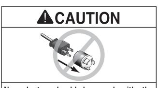
No adapter should be used with the required plug. If the plug does not fit the available receptacle, or the machine must be reconnected for use on a different type of circuit, the reconnection must be made by a qualified electrician and comply with all local codes and ordinances.
